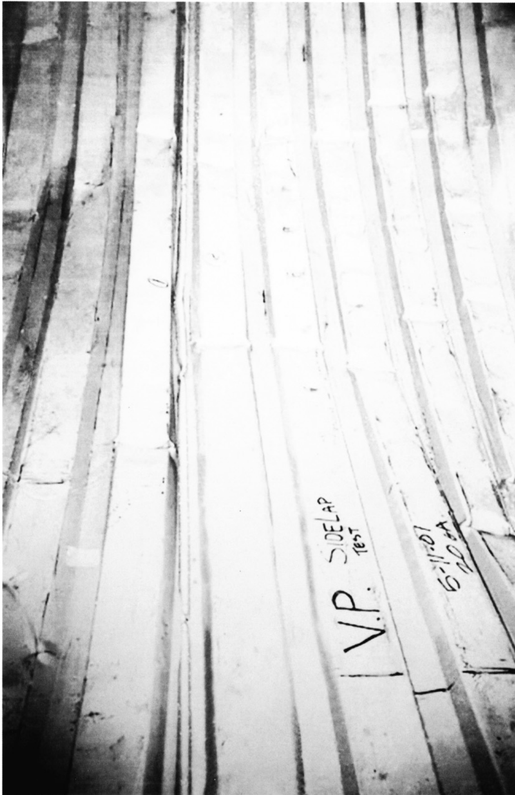
Photo showing the test deck assembly after completion of the load test. Note the compression buckling of the top flanges, which is present on both sides of the side-lap joint. This shows the excellent ability of the PUNCHLOK (tm) to transfer load across the side-laps. At no time during the test or after the test were there any signs of VSC disengagement or slippage.
