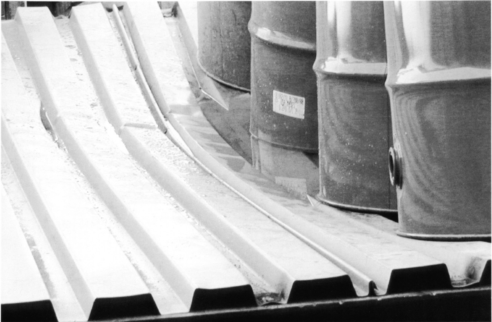
Photo showing the test deck at the load of 120 Lbs./Sq.ft. Note the beginning of compression buckling on the top flanges of the adjacent non loaded sheet of decking. This demonstrates the high load transfer capabilities of the PUNCHLOK (tm) system.
